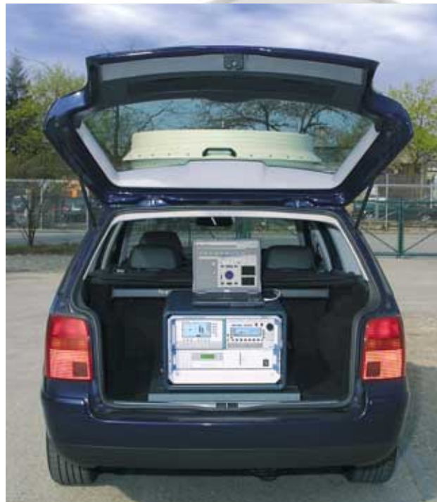
R&S TMS 210 with options, installed in a vehicle
